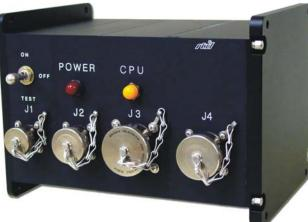
HiDAN*plus*—Integrating the modularity of IDAN with the ruggedization of HiDAN, HiDAN*plus* enables connectors on all system frames, with signals running between frames through a dedicated stack-through raceway.
